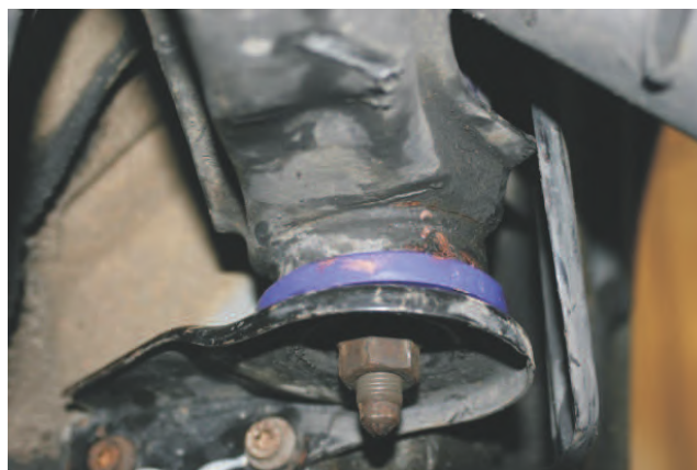
Figure 1 - The assembled rear beam to chassis mount
