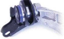
A Bush Inside of car (Supplied washer fits over casting)
