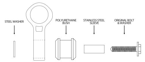
Figure 1: Assembly exploded view
