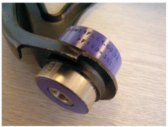
Fig 2: Bush fitted in wishbone
