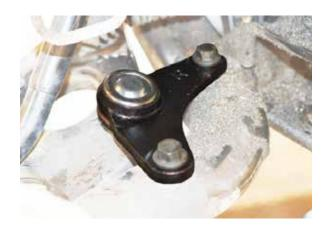
FIT SPACER HERE - Chamfer face inwards so spacer sits flush on the drive shaft. - Flat face towards bearing
