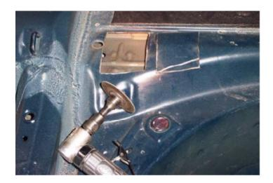
Inside each cutout you will see three rosette welds. Cut a section of the sheet between the three «triangle» welds (see photo below).
