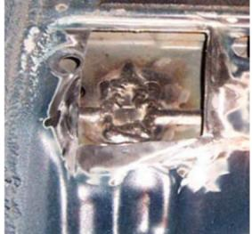
Weld the top sheet to the bottom sheet around the area you just cut out. If you notice cracks in the sheet metal due to chassis fatigue, weld them at this stage. Then clean off the solder residue and burnt paint.
