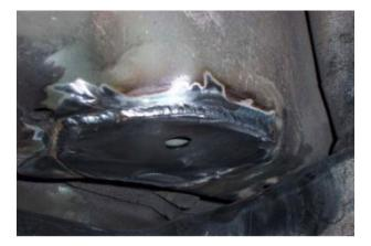
In addition to the welding on the edges of the reinforcement sheet, the small holes allow the stock chassis to be drilled in order to spot weld the two sheets together, always with the aim of strenghtening as much as possible.
