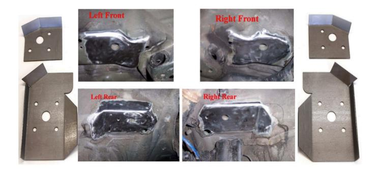
You can use two 12x1.5 bolts to hold the plates in place in the original mounting hole. The bolt does not need to be tightened much as it only serves to align the plate hole with the frame and hold the reinforcement in place during welding.
